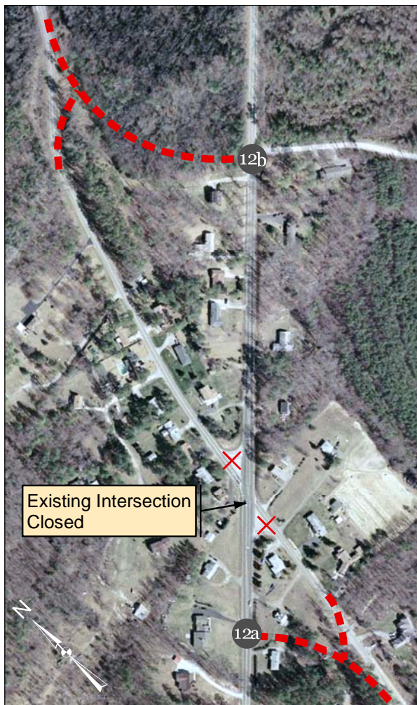
Figure 3-5: Courthouse/Bull Hill Intersection Realignment
